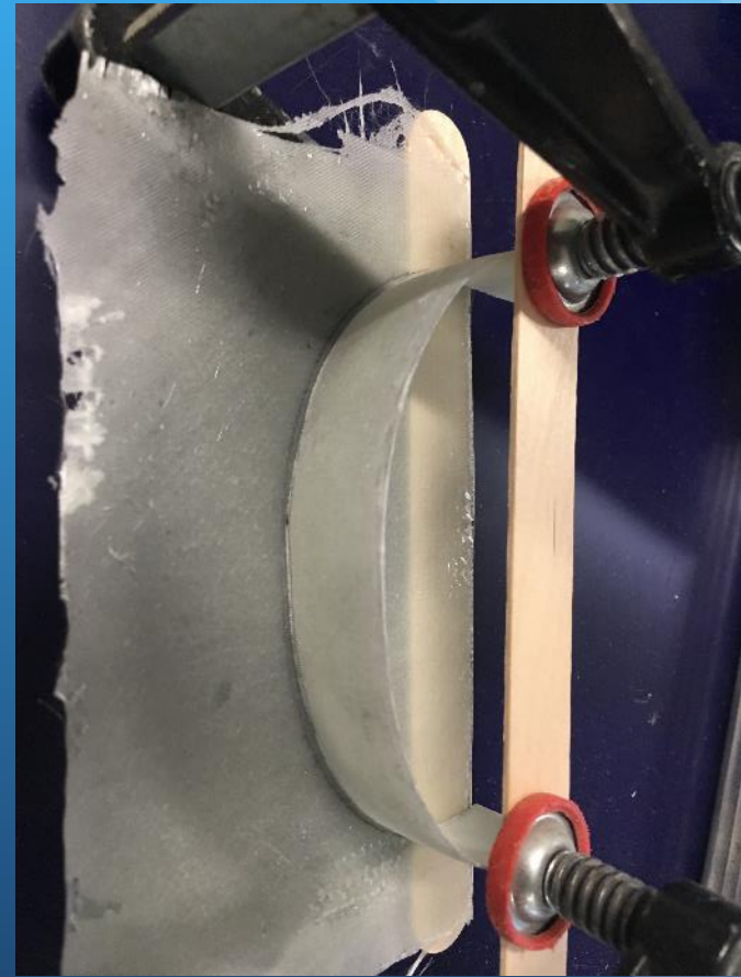
Flange trimmed & set on fillet
