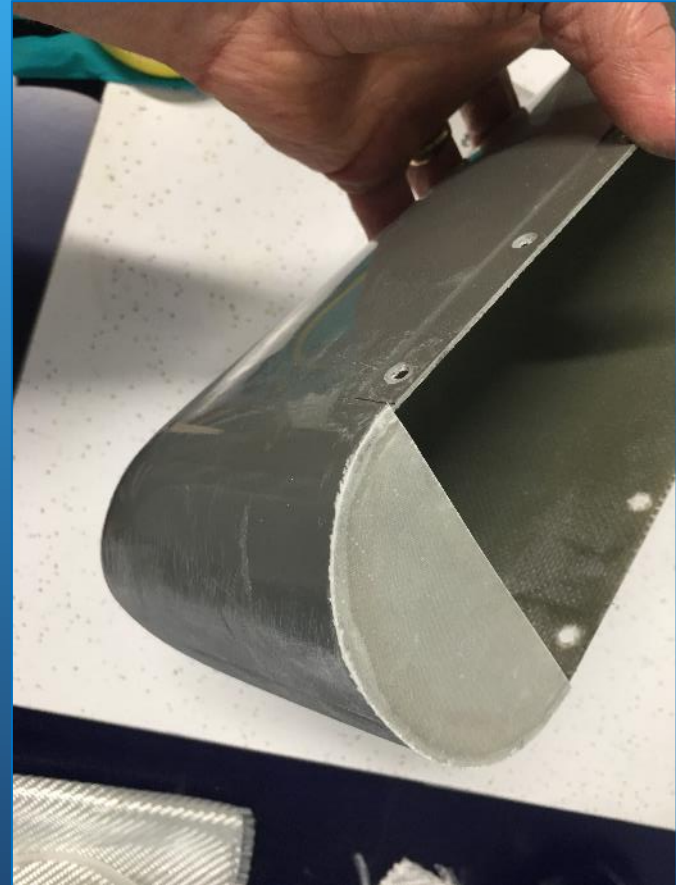
Fillet inserted & glued in place with epoxy
